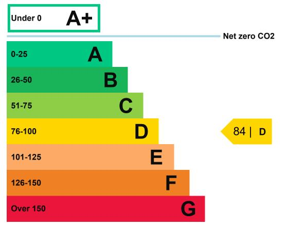
Properties are given a rating from A+ (most efficient) to G (least efficient).
