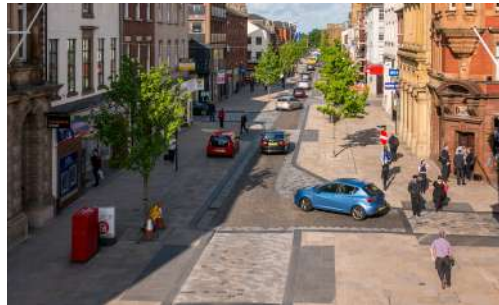
1, 2 Street with flexible space providing short term parking, tree planting, and improved crossing in Preston
