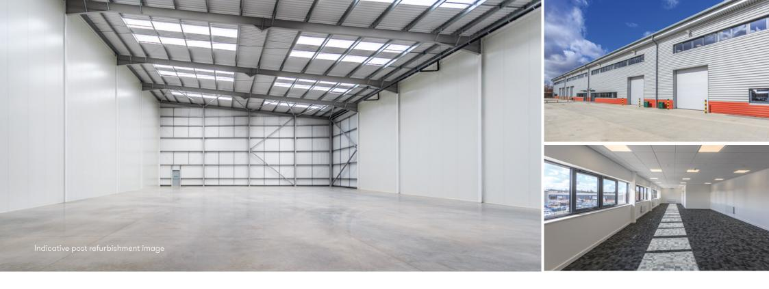
UNIT 2, NEXUS PARK IS A MODERN WAREHOUSE/INDUSTRIAL BUILDING CONSTRUCTED TO A VERY HIGH QUALITY. THE UNIT COMPRISES A STEEL PORTAL FRAME STRUCTURE WITH SHEET METAL CLADDING, PITCHED ROOFS AND FITTED OPEN PLAN FIRST FLOOR OFFICES.
